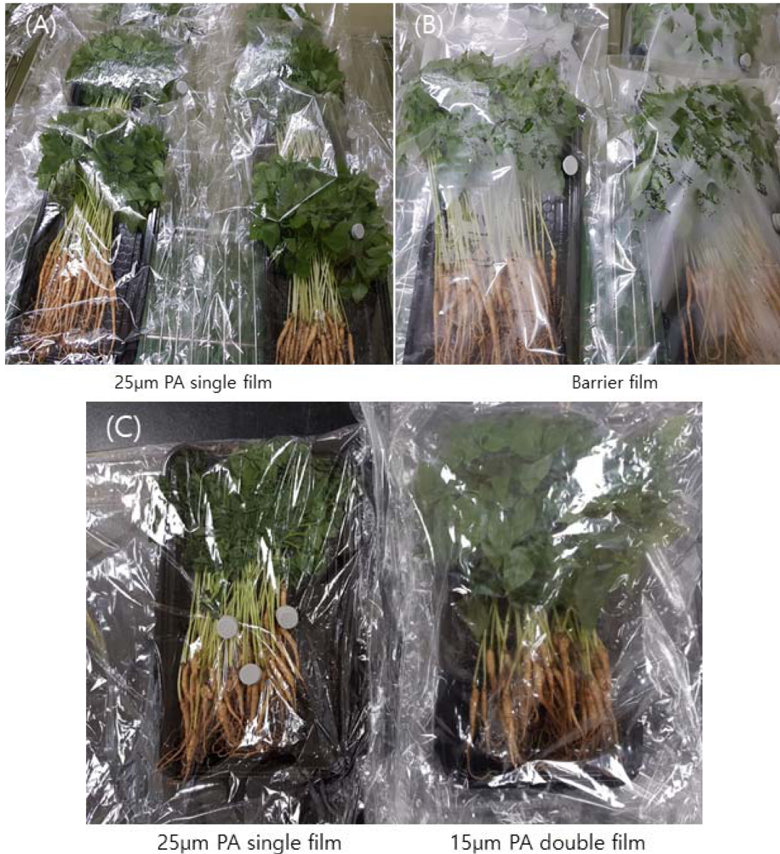
Fig. 5. Appearance of ginseng sprouts packed with PA film and barrier film. (A) and (B); moisture condensation not generated or generated inside the film of ginseng sprouts packaged with PA film and barrier film after storage 2 days at 10°C, (C); appearance of ginseng sprouts packaged 25 \mu\text{m} PA film and 15 \mu\text{m} PA double film after storage 5 days at 20°C.
